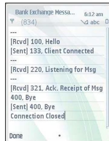
Fig. 3: The screenshot for handshake executed on the cell phone
